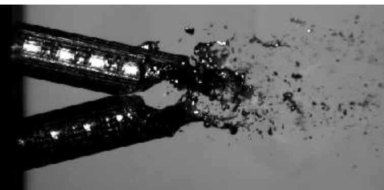
Thermal coating – particle generation in wire arc coating
